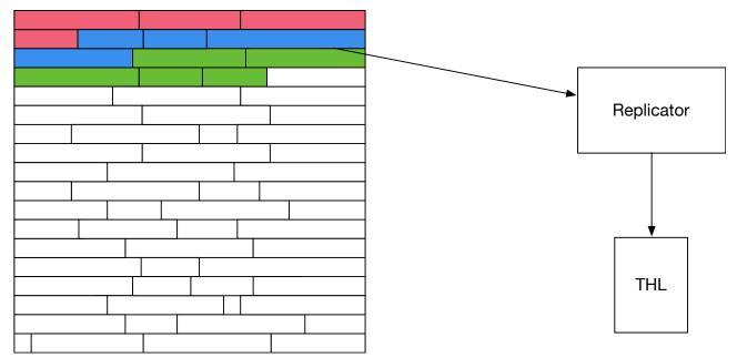
The process of reading the binary log content is constant. Of all the available extraction methods, the MySQL is probably the easiest to understand because it is a simple one-to-one mapping of the source recorded transactional information and the transactions recorded in the THL.
