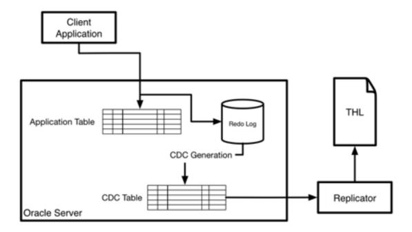
Because continually reading the CDC tables would itself represent an overhead on the Oracle server, the replicator will delay reading if data has not been written for some time. If there have been few changes, it could take up to a minute before the replicator tries to read the CDC tables.
