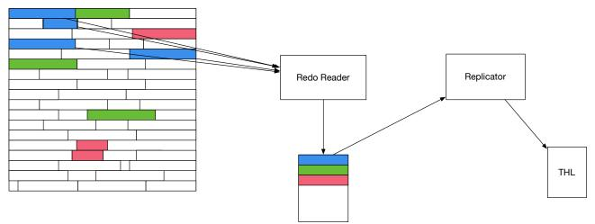
The Redo Reader and Replicator work together to perform the extraction, but also work independently. This means that a redo reader process can operate without the replicator running.
