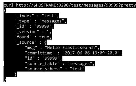
The benefit of replicating data into Elasticsearch this way is that the data can be moved and replicated very efficiently. The use of the REST API in this fashion also opens up the possibility to apply the data into other tools that use a REST API for storing and updating information.
