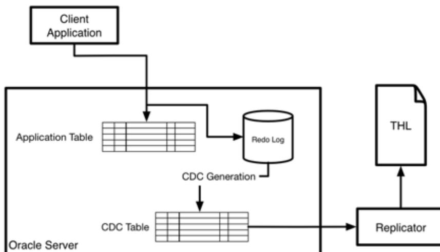
Setting up CDC requires settings within the Oracle database to be enabled and the tables to be monitored configured and added to the CDC process.
